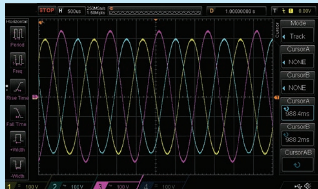
Three Phase Unbalance Voltage Test Captured
